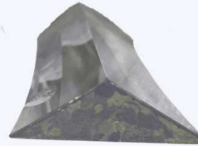
One Prism belonging to the First Order Fresnel Lens from the Cape Fear Lighthouse
